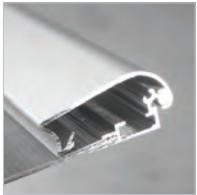
Profile / UYUP007200 1.81" Aluminium Snap profile set (top & bottom) in 118.11" without springs. Top Profile is silver anodized. Bottom profile is mill finished.
