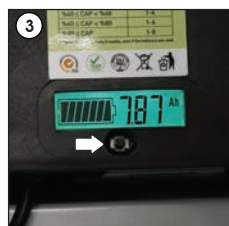
Capacity of battery (0 - 8) Ampere/hour
