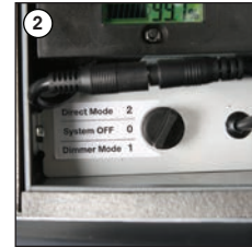
Dimmer Mode 1: Remote control will be activate. The frame works with %50 or %100 bright.
