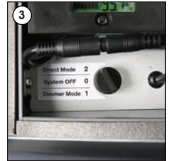
Direct Mode 2: The battery connect directly to illumination. The frame works with %100 bright.
