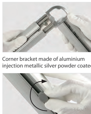
Insert banner buttons into the rear channel of the profile.
